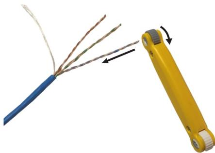
1. Select the appropriate unwinding guide at the end of the tool. Use the smaller guide for CAT 5, 5E, and 6. And the larger guide for CAT 7. Use gentle thumb pressure to turn the guide roller clockwise and simultaneously feed the tool onto the twisted pair.
