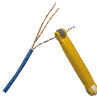
2. Continue turning the guide roller and allow the tool to self feed and unwind the twisted pair.
