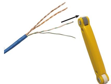
3. Press the guide roller and slide the tool off the unwound twisted pair to straighten them.
