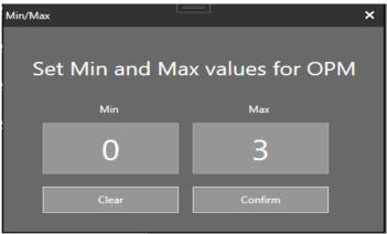
Loss minimum is usually set to 0. A maximum of 3 is standard for most fiber tests. Set Min and Max to any values as needed, then click "Apply".
