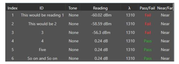
Any readings which fall within the Min/Max range provided will be given a PASS designation. Readings that do not fall within the range will be given a FAIL designation.
